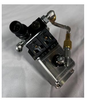
Start by removing the black thumb nuts on each of the solenoids. Be careful, behind each one is a small o-ring. These will need to be removed as well. Be careful not to tear, knick, or break this o-ring, as it will need to go back on later. Once removed, slide the solenoids off of each post and set aside.
