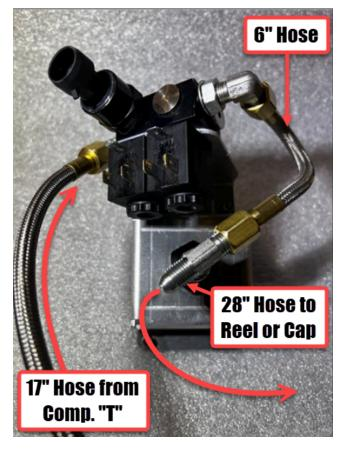
If you purchased your TAC System with the APEX hose reel, the other side of the "T" is the "Out to Hose Reel" port. This is where the 28" Braided steel air line will connect. If you did not opt for the reel, simply leave or install the 90\* fitting (instead of the "T"), that came with the basic TAC System, in this location.
