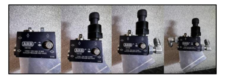
**Note -** The 90\* fitting is equipped with a small non-removable flat washer. This washer may make contact with the cap/plug directly next to it. It may be necessary to file a flat on the edge of the washer to clear the cap. Not doing so may result in an air leak later on.
