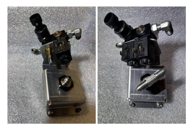
Install the 6" braided air line between the "T" and 90\*BSP fitting as shown below. Once fitted, tighten the fittings. *Make sure not to kink hose.*
